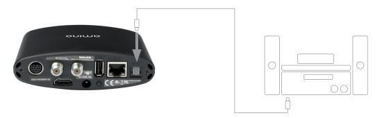
Connect an optical S/PDIF cable to the S/PDIF optical output of the A140 and the S/PDF optical input of an AV amplifier or home cinema system.
