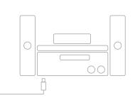
Connect an optical S/PDIF cable to the S/PDIF optical output of the A540 PVR and the S/PDF optical input of an AV amplifier or home cinema system.
